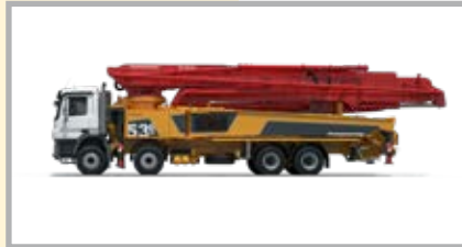
Concrete pump M53
